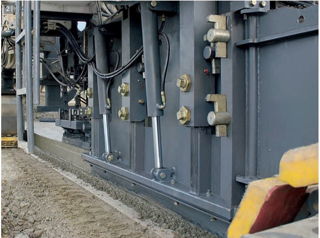
2 | Hydraulically adjustable side-plates ensure clean concrete edges.
