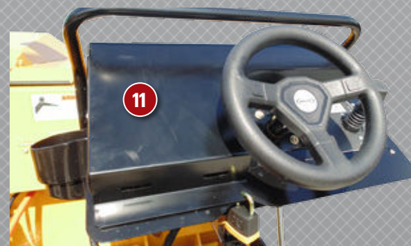
Lockable vandalism covers and engine access doors provide security.
