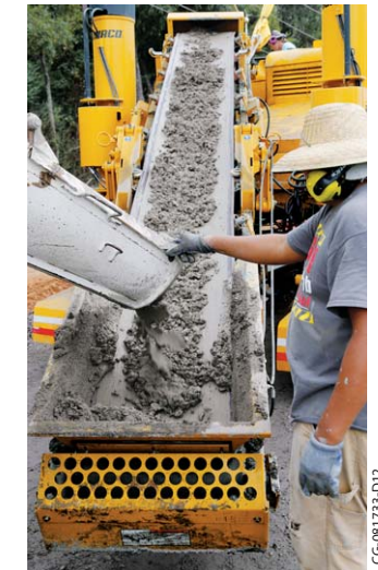
The folding conveyor features four-way hydraulic positioning for optimum concrete delivery and placement.
