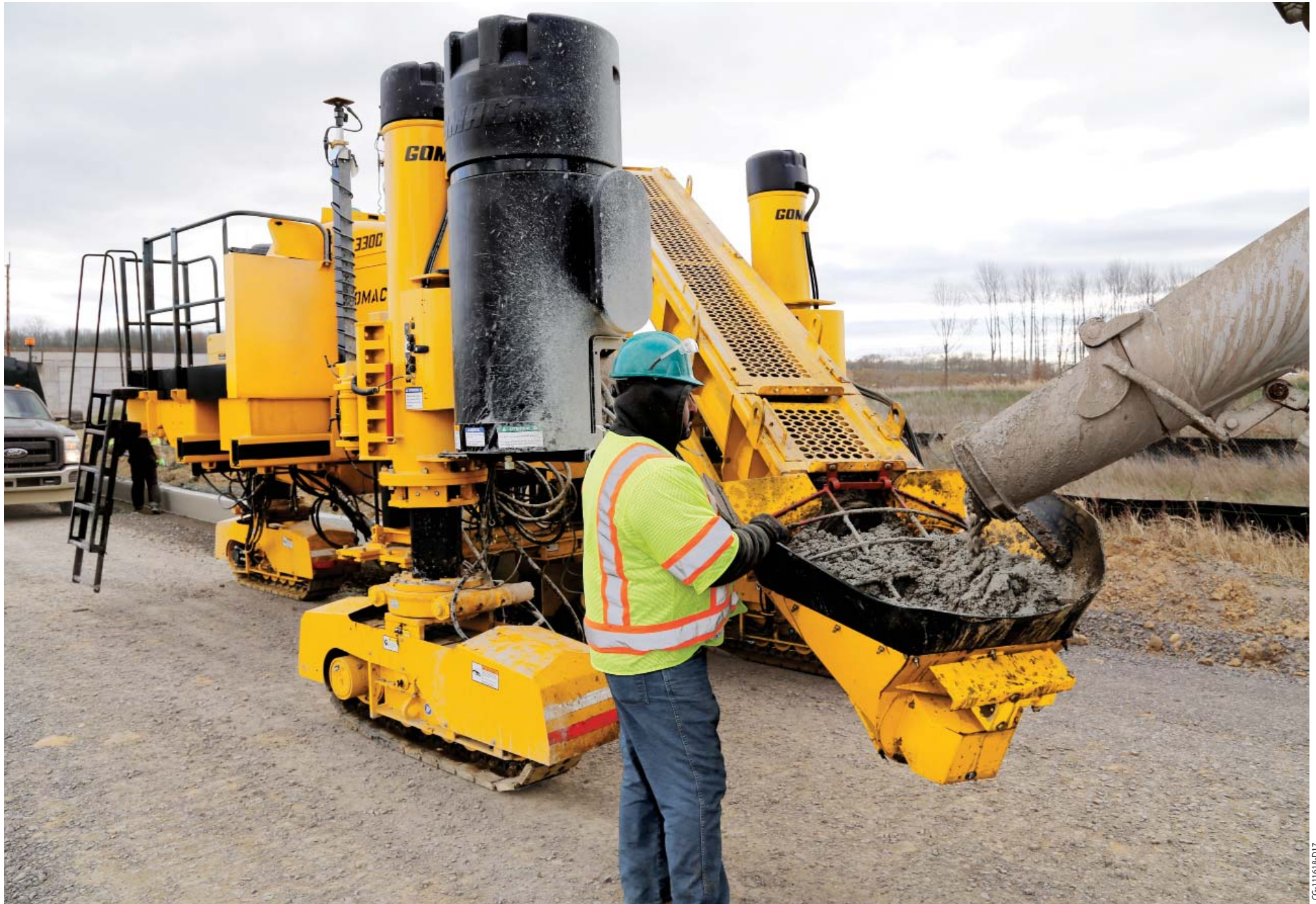
The charging auger on the 3300 is equipped with vibration to release concrete build up from the safety guard at the end of the hopper. The auger's safety guards are hinged to allow for cleaning.
