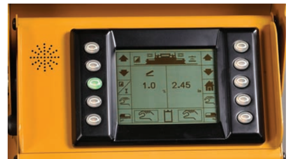
Cat Grade and Slope Control
