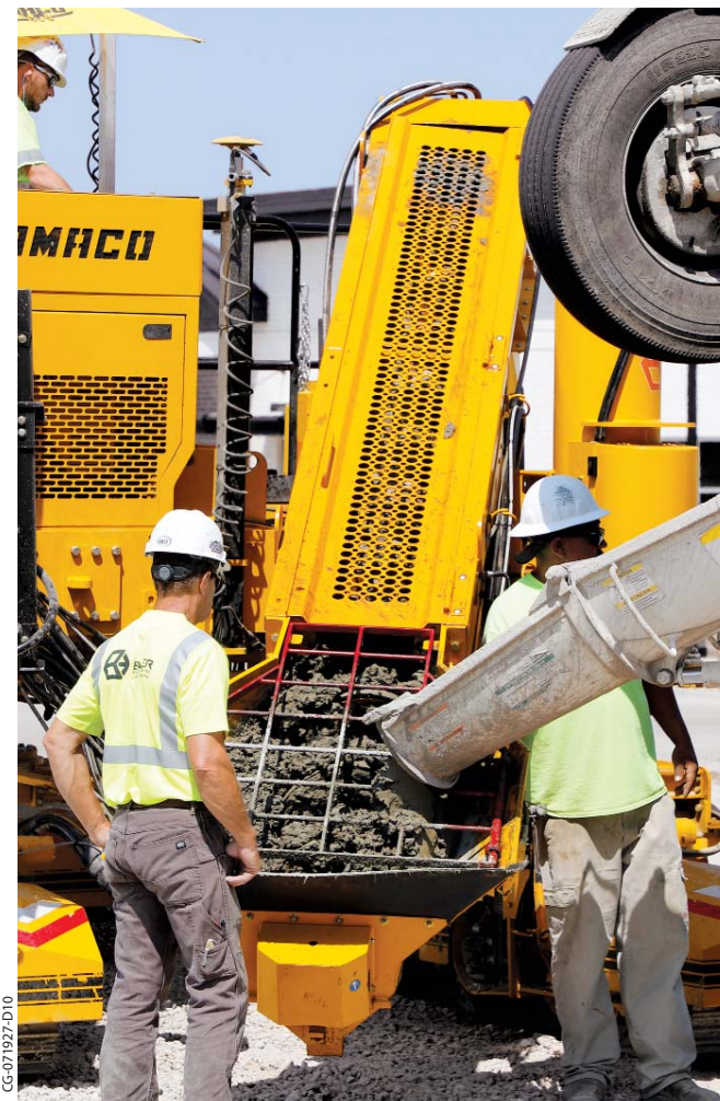
The optional 17 foot (5.18 m) long hydraulically driven auger is equipped with vibration to release concrete build up from the safety guard at the end of the hopper. The auger safety guards are hinged to allow for cleaning.
