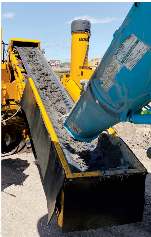
The 16 foot (4.88 m) long, 24 inch (610 mm) wide conveyor can move the concrete into the hopper at a speed of up to 284 feet per minute (86.6 mpm).
