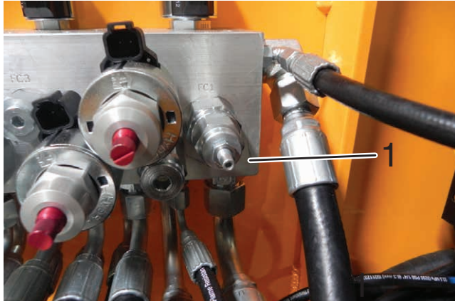
Generator Flow Control Adjuster
