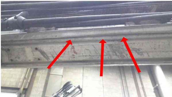
Slide cover take off and dirt underneath
