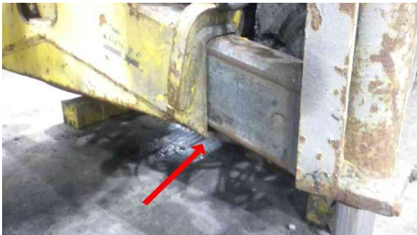
Outrigger need to be rebuilt,loose
