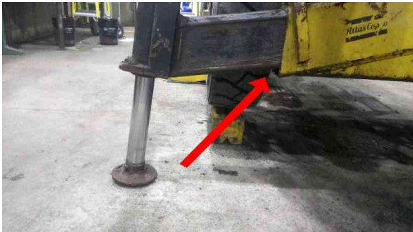
Right outrigger loose,tefflons haves to be replace
