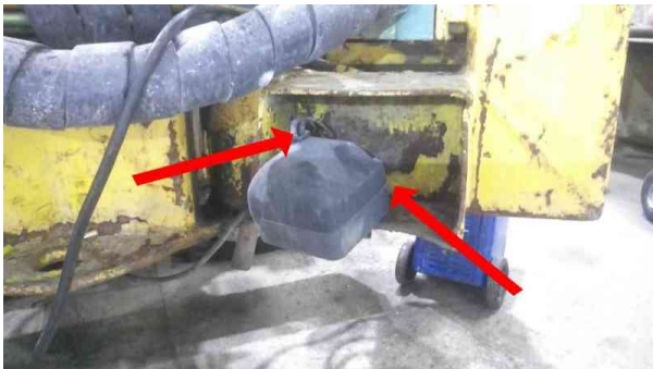
Rear right light broken
