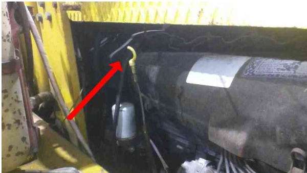
Engine dipstick broken, Engine #F5L912W S/N:8740752
