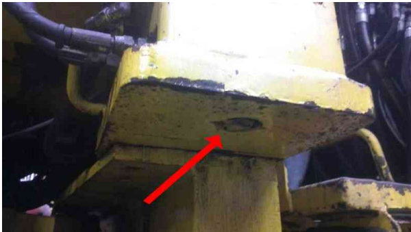
Lifting cylinder right side is leaking
