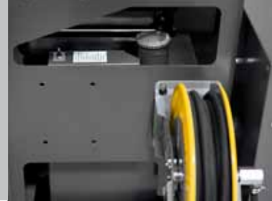
Emulsion spray system
